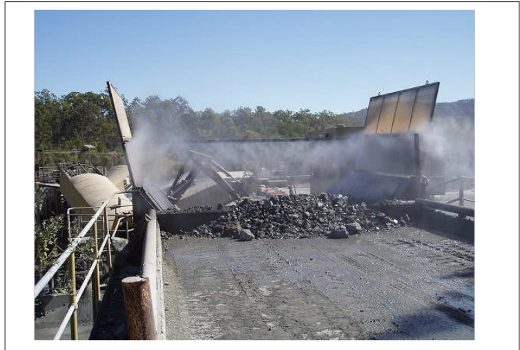
Dump bin fog curtain from a different angle; the curtain is usually only activated during transfer.
